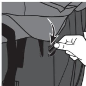
4. Push the anchor down through the new slot to the bottom of the seat (A) then feed it through the original slot to the top of the seat (B) and repeat for other side.
